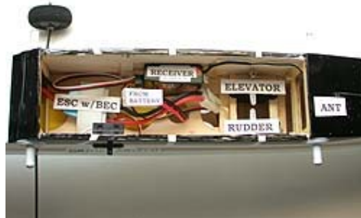
All components installed inside the fuselage in the area under the wing. The white connector, just to the right of center, is the battery connector that goes to the ESC.
