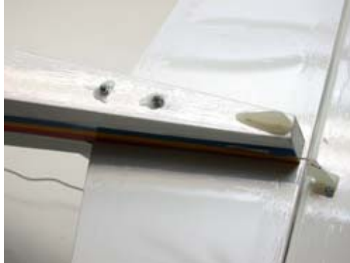
The rear fuselage underside. The two nuts that hold the vertical fin and stab in place can be seen in this photo. Also shown are the tail skid and the elevator control horn.
