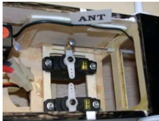
The rear portion of the RC compartment showing the rudder and elevator servos plus the receiver wire antenna. Keep the antenna away from the servos as they may interfere with radio command reception.
