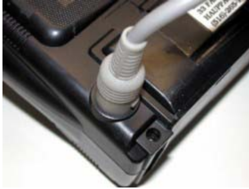
Rear of Radiant; trainer cable is plugged into special jack. Same goes for other transmitter, which gets other end of cable.
