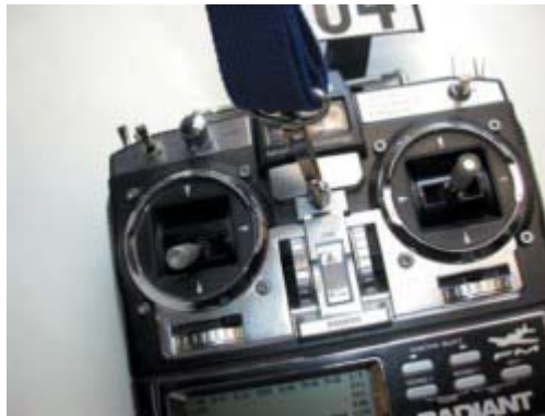
Transmitter neck strap attached to hook and eye on Airtronics Radiant transmitter. Strap goes around pilot's neck and supports transmitter case, leaving both hands free to grip and operate transmitter control sticks.
