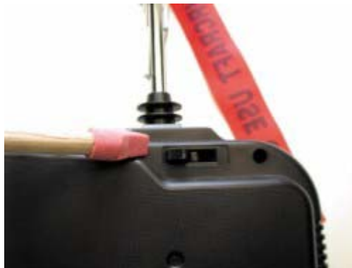
Rear of Hitec three-channel transmitter showing throttle channel lever located away from case edge, which would be the idle position.
