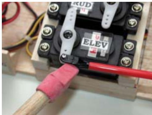
Pointer shows black plastic keeper that prevents control-rod wire end from falling off servo output arm. Output arm screw is securely in place. Without this screw, servo output arm might fall off. Which hole you select on servo output arm affects amount of control throw obtained.
