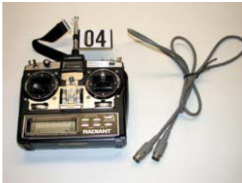
Airtronics Radiant transmitter (L) and trainer cable used to connect two RC transmitters. Student holds one transmitter and instructor holds other. Instructor can hit switch and take primary control of model at any time.
