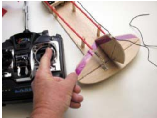
Finger holds rudder-control stick over on transmitter, and rudder is hard over at aircraft (mock-up) end. It means rudder is moving in correct direction; applying right rudder at transmitter results in right rudder at aircraft.
