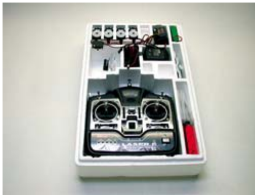
Typical RC system—Hitec Laser 6 (six-channel function transmitter with four servos)—as it arrives in Styrofoam shipping container. Transmitter is at bottom; four servos are at top. Included are receiver, battery charger.
