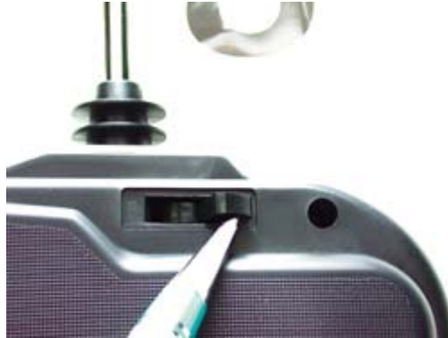
Pen points to third channel lever, on rear of Hitec three-channel transmitter. Index finger of left hand moves this lever. It controls engine speed (throttle control).
