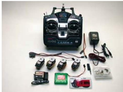
Hitec RCD Laser 6 is full four-channel RC system—a step ahead of basic or beginner's radio. Transmitter has six-channel capability; receiver has at least six channel functions. System comes with four servos to cover four basic flight-control functions. It costs less than $200 and will serve well for many years as you progress from beginner through expert.
