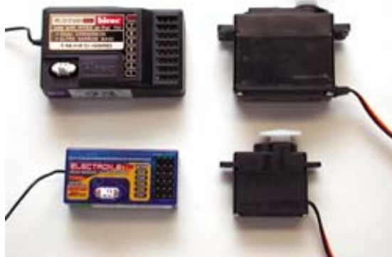
Comparison of RC receiver, servo sizes. Top left: Hitec RCD eight-channel receiver capable of controlling models up to large sizes— 1/4 scale and up. Top right: Typical- or average-sized Hitec HS-422 servo can easily control models with up to 60-size glow engines. (These are components from Hitec Laser 6 system.) Bottom left: Hitec Electron 6 receiver weighs slightly more than 1/2 ounce! Companion miniature HS-81 servo is at bottom right. This receiver, servo is ideal for smaller glow-powered models and small electric park flyers. (These components are from Hitec Neon three-channel FM RC system.)
