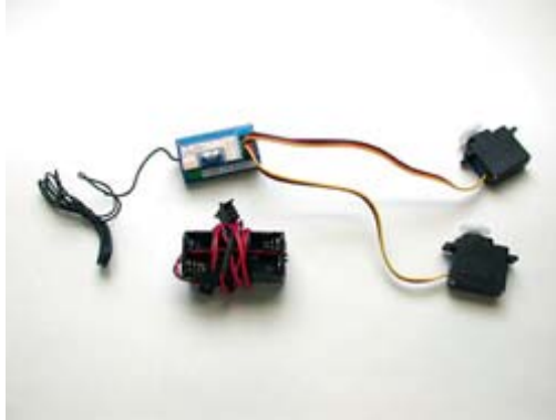
Hitec Neon three-channel FM airborne components (that go inside model). Receiver is at top; below is four-cell battery box intended for nonrechargeable alkaline cells; two HS-81 miniature servos are at right. This type of lightweight RC system is intended for small glow-powered models (.049-.15) and park-flyer electric-powered models.
