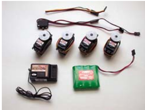
Typical four-channel airborne RC system goes into average- to larger-size model. Top: Aileron extension cable, switch harness, four servos. Bottom left: receiver. Bottom right: four-cell Ni-Cd rechargeable battery pack. Components weigh roughly 12 ounces; will fly 20- to 60-powered and medium to large electric-powered models.
