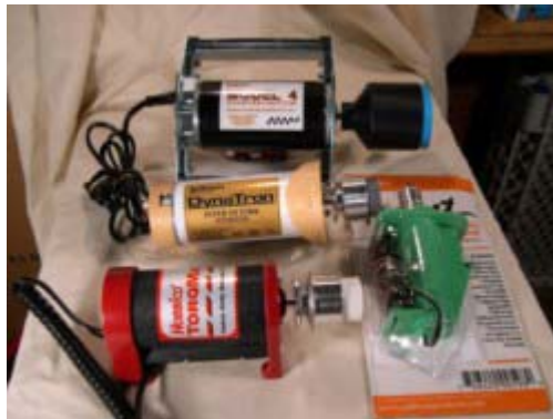
Photo 5 – A starter for every model engine. 12-volt red/black Hobbico standard-duty is best on engines up to .90 cu. in. The 12/24-volt, gold/white Sullivan Super Hi-Tork heavy-duty is designed for all engines up to 2.35 cu. in. The Black, 24-volt Model 4 Sullivan starter is for up to 24 cu. in. gasoline motors. There is even a starter for 0.49 size engines, the green Sullivan Hornet. (Photo courtesy of Hobby Hut, Pompton Plains, NJ)
