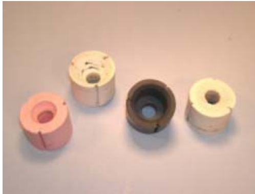
Photo 6 -- The pink starter insert is designed for engines equipped with AMA safety nuts. The white insert fits most common spinners up to three inches. The dark gray insert fits sharp, deep cone spinners and larger spinners. When reversed, all inserts will fit small AMA safety nuts or engines without spinners or safety nuts.
