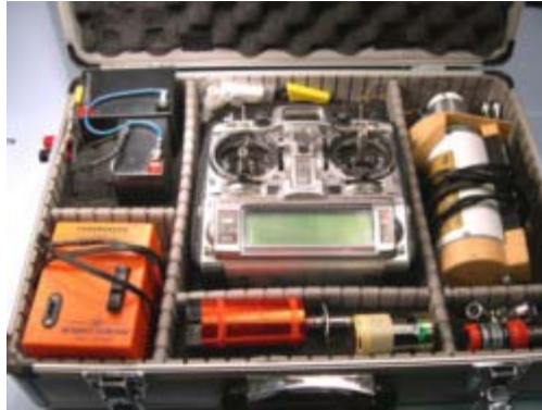
Photo 3 – A competition flight line starter case. The two small batteries provide 18 volts for a positive start every time. The orange Radio South Glow Igniter automatically adjusts the current flow to light the plug under all conditions. Backup glow igniters are also available including one that uses an alkaline "D" cell for power.
