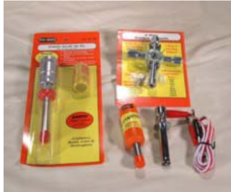
Photo 10 – The Du-Bro glow plug igniter on the left features a rechargeable and replaceable Ni-Cad. The orange McDaniel Ni-Starter has a meter to let you know if the plug is bad. The cord and plug igniter are typical of those used with a power panel. A good glow –plug wrench is invaluable.
