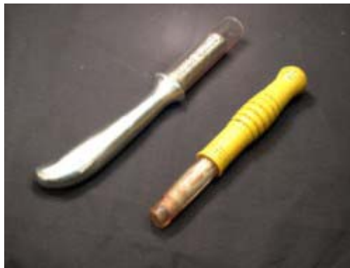
Photo 9 – The two most common chicken sticks. J’Tec’s all-metal Power Stroke looks sharp and works well, but costs $11. The $5, well-used, wooden SonicTronics Cheeter Stick works just as well but is not very fancy. Either one will prevent those hospital “stitch up” visits that tend to spoil many flying sessions.
