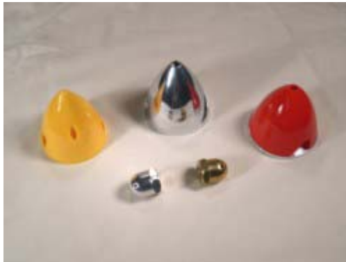
Photo 7 – The two small Harry Higley AMA safety Nuts meet AMA insurance requirements and look nice on aircraft like Piper Cubs, P-47 Thunderbolts and B-17s. The brass nut weighs 2 oz. and is used to add nose weight. Sharp spinners like the yellow or metal work best with the pink insert. Standard spinners use the white insert. (Photo courtesy of Hobby Hut, Pompton Plains, NJ)
