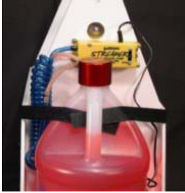
Photo 4 – A typical position for the electric fuel pump. Having the pump close to the plastic, not metal, fuel container reduces the pumps workload. This Sullivan Streamer pump has its own switch, but will also work using the power panel’s switching. Some pumps do not have internal switches and require a panel to operate.
