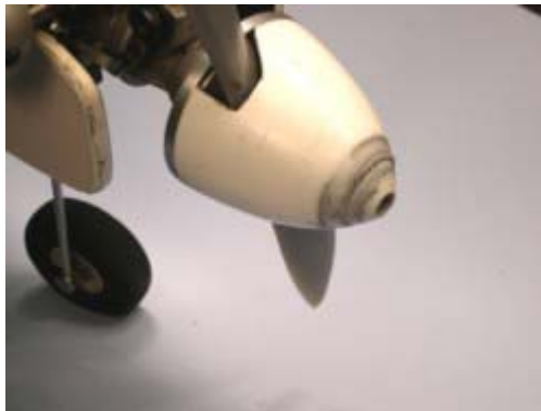
Photo 8 – A starter has damaged this spinner. Always hold the starter cone tight against the spinner before turning it on. If the starter must rotate before contacting the spinner, either the field
