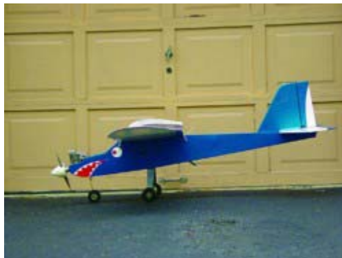
A good ground stance has the wing sitting at a small but positive angle of attack: somewhere between 0° and 3° positive.
