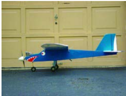
A good ground stance has the wing sitting at a small but positive angle of attack: somewhere between 0° and 3° positive.
