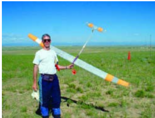
Pete McQuade with his high-tech F1A Towline Glider. Modern F1As feature a “bunt” transition following a zoom launch; both aid in height gain.
