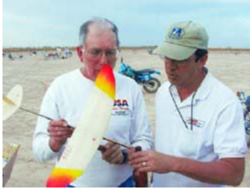
Above and below right: Expert Glider flier Lee Hines shows the details of his legendary Sweepette HLG, originally designed in the late 1950s and still competitive. Little black rotary gadget is a lightweight DT timer. After two minutes the spring tension on the timer releases the line holding down the wing, which then hinges back abruptly, parachuting the model to the ground.
