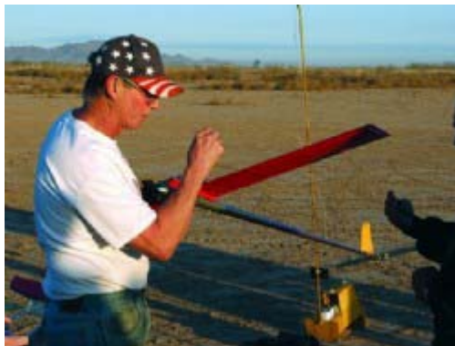
F1C flier Ed Carroll prepares for an early-morning flyoff with his Russian-built folding-wing model. Folders are finally gaining a foothold in F1C competition after years of experimentation. The advantage of a folding wing is less drag during the rapid climb phase.
