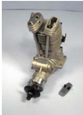
O.S. 120 valve and rocker arm assembly is visible with valve cover removed. Thin tubes in front house pushrods that operate valves.
