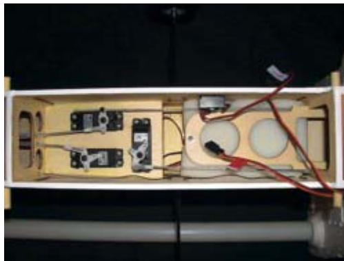
Servos in place after reinforcing mounts. Author has had three servo screws strip mounts without using reinforcement.
