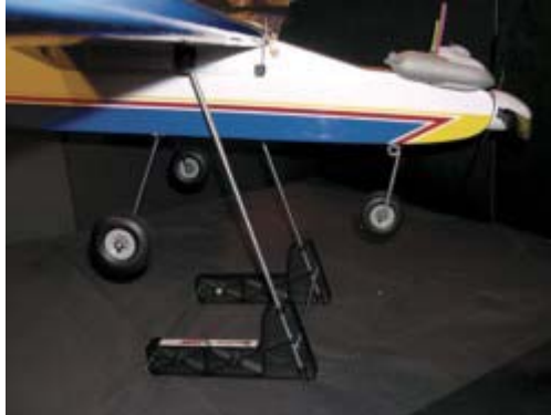
Hangar 9 Arrow on Great Planes C.G. Machine. Stand allows positioning test weights and immediately checking effects. CG is correct when nose points downward roughly 10°.
