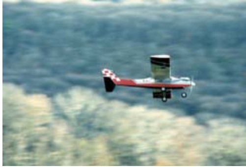
Midwest Aerobat is outstanding flier with semisymmetrical wing. Twin aileron servos allow computer transmitter to use ailerons as flaperons for extra lift, speed reduction, and amazing attitude changes when coupled to elevator.
