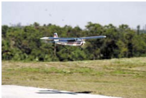
Hobbistar 60 Mk III uses slightly semisymmetrical airfoil, but its overly large 875-square-inch wing area makes up for any missing lift. Its airfoil does improve inverted flight performance. Photo courtesy Ron Farkas.
