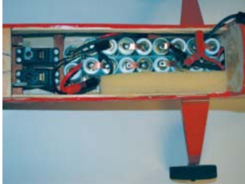
How the Acrovolt's crowded battery compartment looked when Bob had to employ upward of 18 3000 mAh NiMH cells.
