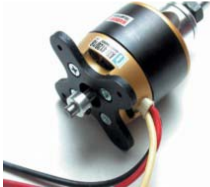
Closer look at AXI 4120/18 motor from rear shows accessory radial mounting plate which Bob highly recommends. Collar on shafts moves up flush with rear of motor.
