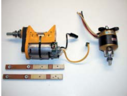
L-R: Older, larger, heavier DeWALT motor with H-1000 belt drive and replacement Hobby Lobby AXI 4120/18 brushless outrunner motor. It weighs 11 ounces!
