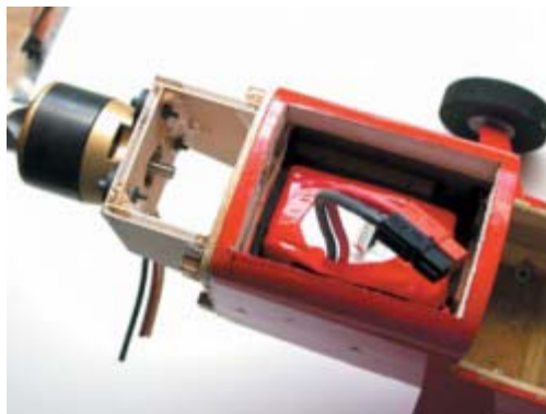
Upper view shows added plywood motor box and battery-pack position. Jeti brushless ESC is also in battery compartment.
