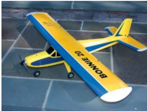
Bonnie 20 electric-powered ARF is featured in Sport Aviator review. It could have been powered by .20-.32 glow engine. It also makes a wonderful electric-powered advanced RC trainer.
