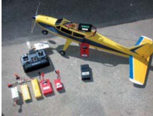
Using Whattmeter to take motor data of electric power equipment in Hobby Lobby Bonnie 20, note battery packs lined up in foreground for test purposes. In front is TNC tachometer for measuring propeller rpm.
