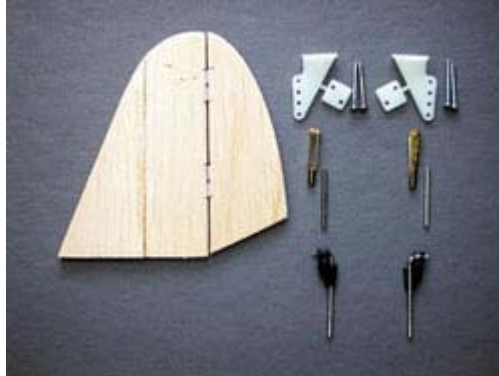
Vertical fin and rudder shown hinged. At right is typical control-hookup hardware: control horns (top), clevises and threaded adjustment rods (center), wire and keeper that attach to servo output arms (bottom).
