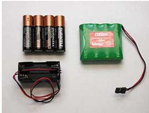
Four-cell airborne battery box (left) holds AA alkaline cells. Typical four-cell Ni-Cd rechargeable battery pack is on right.
