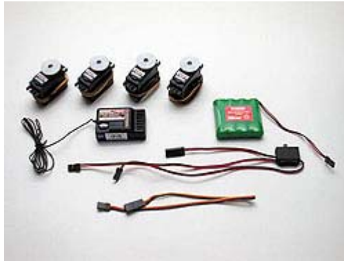
Components supplied with Laser 6 system: four servos (top left), receiver (middle left), battery pack (middle right), switch harness (below pack), aileron extension cable (at bottom).
