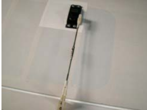
Completed wing-servo and linkage installation is aerodynamically clean and looks good. Short, direct control rod provides positive aileron control.
