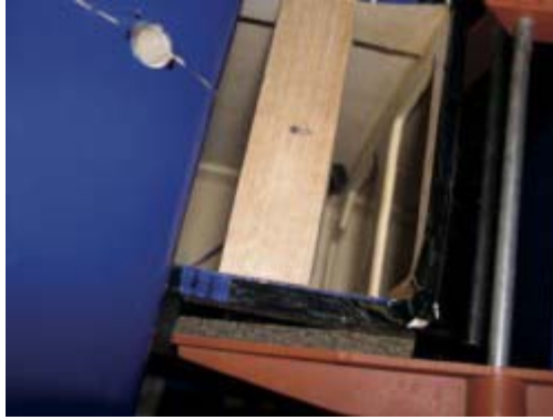
Front maple block is epoxied in place. Make test mark by passing pencil through wing's front arrow shaft once wing is measured and properly positioned.
