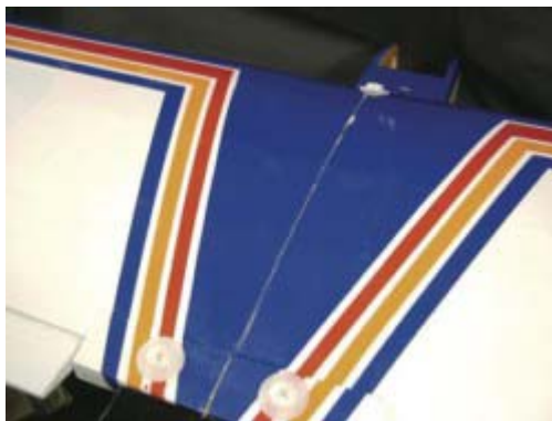
Completed bolt-on wing installation seen from top before covering center seam with trim covering. This strong mounting system maintains flight trim from one flying session to next.
