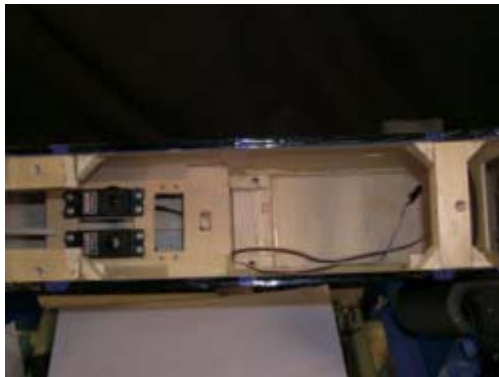
Completed fuselage part of bolt-on system. Note 1/2-inch triangle stock "reinforcers"
