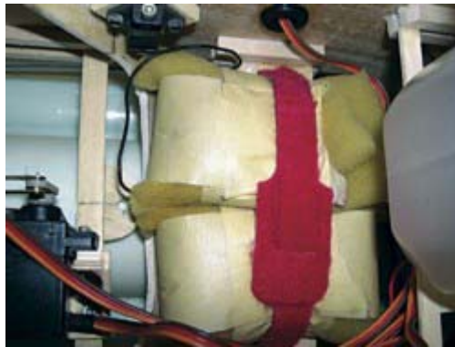
Well-padded, receiver and battery nestle together under hook-and-loop tie wrap. Tighten wrap securely, but don't crush foam, or its padding will be ineffective.
