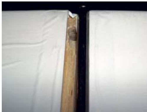
Relieve some wood from landing-gear hole in fuselage as shown. This allows wire gear to rest flat in slot as also shown.
