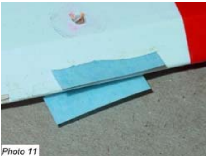
PHOTO 11 - Bracing a control horn position
