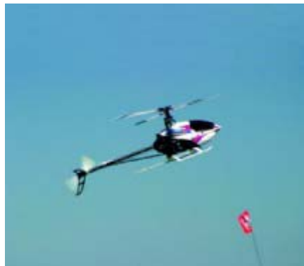
The Hirobo Lepton EX is MRC's latest offering in a 30-size electric helicopter. It uses CCPM mixing and single-piece carbon-fiber side frames.
