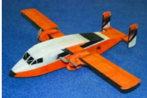
Jason Noll, with his father Frank (Frank's model shown), designed and built a pair of Shorts Sky Vans from 3mm and 6mm Depron. A pair of RimFire motors fly this 11-ounce model.
