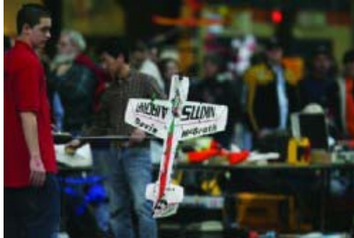
Devin McGrath demonstrates just how “locked” his Nikitis Animal is in a hover; he needed only rudder and power to maintain position.
