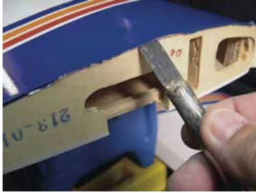
Lifting overlapping covering and trimming it back strengthens wing's center joint by allowing full wood-to-wood contact.
