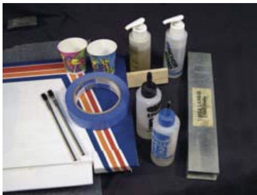
Twelve- and 30-minute epoxies, mixing cups with epoxy brushes, and low-tack masking tape with elasticity glue will be needed to glue wing halves together.
