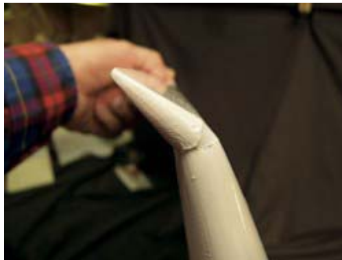
Aileron is deflected 45°-50° during installation. Larger deflection allows flaperon use but causes unacceptably large 1/16-inch gap between wing's TE and aileron. This must be fixed.
