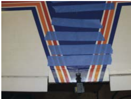
Stretch the tape while applying it. Tape both sides of the wing. The rear clamp ensures TE alignments.
