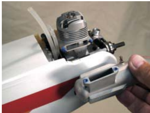
Apply removable thread-locking compound to muffer holes and bolts. Do not use permanent type; that will prevent removal.
