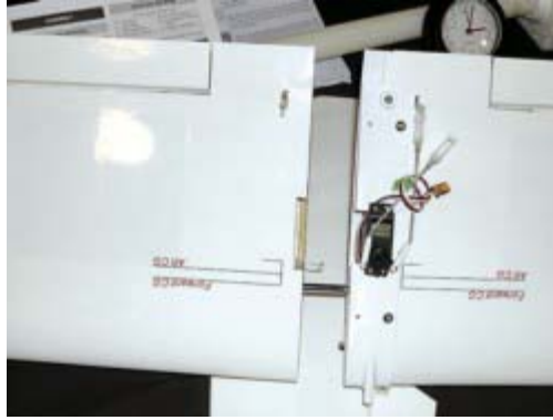
The Hobbico NexSTAR employs solid-steel rods to join wing halves and a full-length plastic center rib for alignment.
