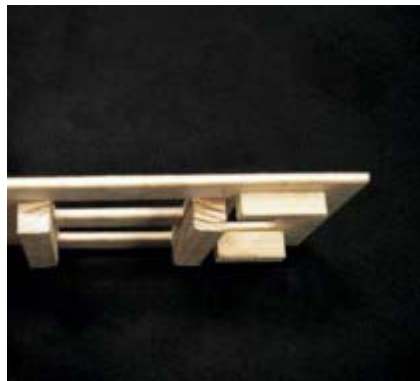
Large \frac{1}{2} \times \frac{1}{2} spruce was used for photo purposes. Thinner \frac{1}{8} \times \frac{1}{2} strips are lighter and easiest to install. Reinforce aileron mount as well.
