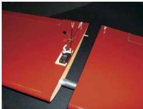
The Hangar 9 Alpha-series RTFs use light aluminum tube spars and a rear alignment pin to join the wing halves.
