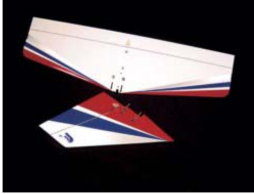
Hangar 9's Alpha 60 employs two bolts to mount the fin and stabilizer and two more to bolt the assembly to the fuselage.
