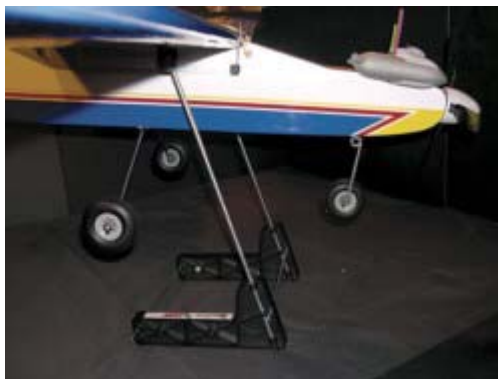
Hangar 9 Arrow on Great Planes C.G. Machine. Stand allows positioning test weights and immediately checking effects. CG is correct when nose points downward roughly 10°.
