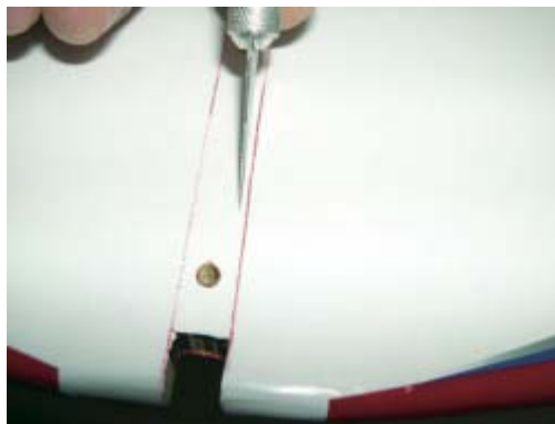
Using a sharp blade, gently cut \frac{1}{16} inch inside the lines but not into the wood. Remove covering before gluing in place.
