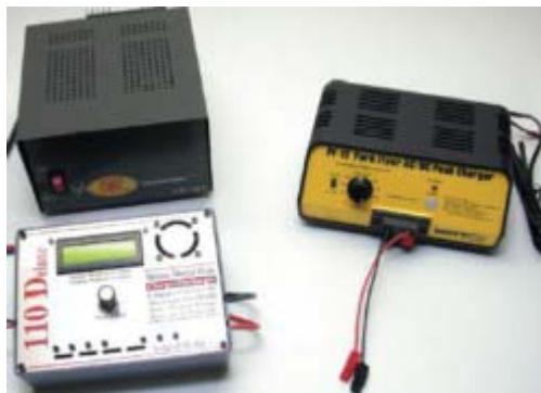
Watt-Age charger is capable of operating at home on 115VAC and at flying field off of 12-volt DC car battery. The 110 Deluxe requires separate 115VAC to 12VDC power supply (at rear) to operate from home shop.
