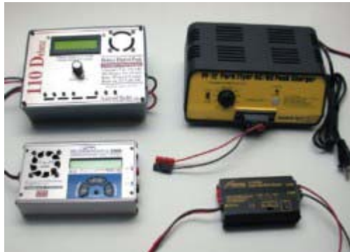
Popular field-type fast battery chargers. Clockwise from top left: AstroFlight 110 Deluxe, Watt-Age PF-12 Park Flyer AC/DC Peak Charger, tiny Dymond Modelsports four- to eight-cell mini-peak charger, FMA Direct Super Nova automatic peak-detect charger. All employ peak-detect-type circuitry—as it should be!
