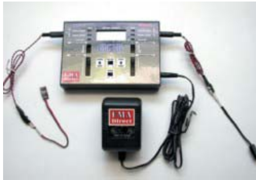
FMA Direct Einstein XL dual-output battery discharge tester/cycler (at top) and 115VAC power supply for it.
