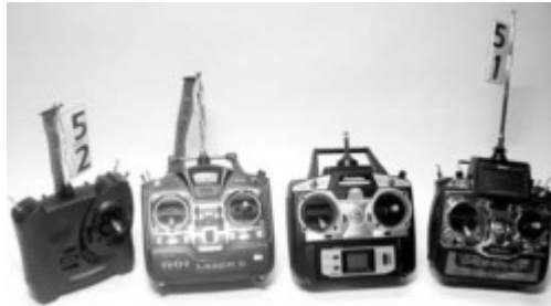
Typical RC transmitters (L-R): Hitec Neon three-channel (single control stick); Hitec Laser 6, which has two control-stick assemblies but is basic—not a computer radio; Futaba T6EXA entry-level computer radio; Hitec Eclipse, which is computer driven and has channel synthesizer.
