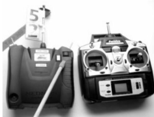
Left: Rear of Hitec Neon three-channel single-stick transmitter. Pointer shows location of throttle-control lever which must be moved side to side to adjust engine/motor speeds. Right: Futaba T6EXA computer transmitter, which has two control-stick assemblies. Throttle control is obtained from left stick and operated in up-and-down movement (for high and low throttle settings).
