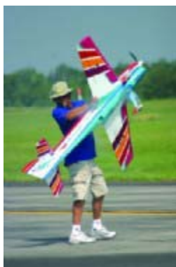
Jason Shulman carries Sean McMurtry's Astral XX to the runway. The anhedral stabilizer offers more finite control in FAI-class rolling maneuvers.
