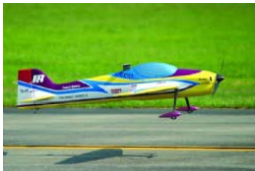
Quique Somenzini found that the addition of the fixed fin behind the canopy of his RC Aerobatics model made a positive difference in side-area control performance.
